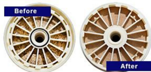
Figure 1: Membrane Module Before & After Cleaning
